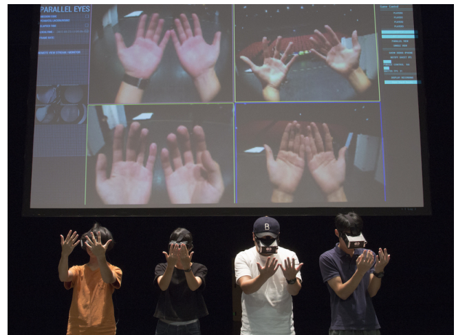
Figure 1. Parallel Eyes: a technology probe for creating a mutual visual shared parallel experience. With Parallel Eyes, users wear a head mounted display which shows shared videos of each other's perspectives as well as one's own perspective in realtime.
